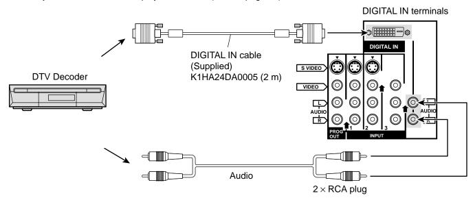
By inputting a High-bandwidth Digital Content Protection high-definition picture source to the DIGITAL IN terminal of this television, high-definition pictures can be displayed on the screen in their digital form. (This terminal is for use in the future when High-bandwidth Digital Content Protection DTV decoders, DVD players and D-VHS are put on the market.)
