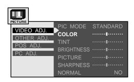
Press to adjust the desired level by looking at the picture behind the menu.
