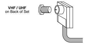
**Cable Connection -** For reception of cable channels (01 - 125) connect the cable supplied by your local cable company. Antenna Mode must be set to CABLE. (Refer to Antenna Mode section.)
