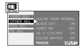
When the screen is single, press TV/VCR to freeze the screen.
