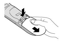
2. Install the batteries as shown in the battery compartment. (Polarity + or – must match the markings in the compartment.)
